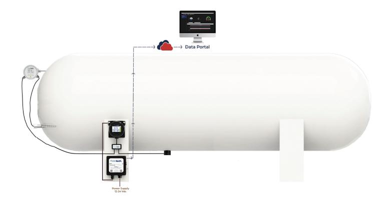
Our products are all seamlessly connected to our Secure Online Data Portal via our ATEX/IECEx certified telemetry device (RotoHub).
