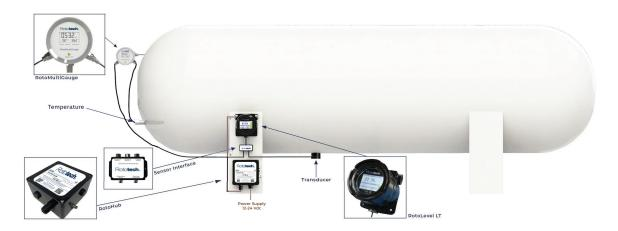
The RotoMultiGauge also forms part of an innovative high technology solution for controlling the inventory of a storage tank. When integrated with our ultrasonic level measurement device (RotoLevel LT) and telemetry device (RotoHub), the user is able to manage and control their tank inventory via our secure online DataPortal.
