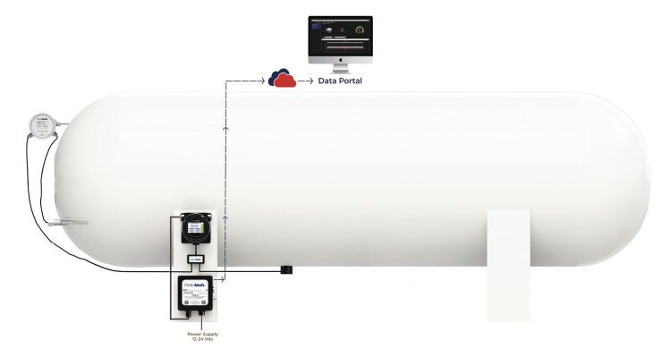
To enable full inventory control of your storage tank, The **RotoMultiGauge** can be seamlessly connected with our certified **RotoLevel LT** device (non-invasive ultrasonic level measurement) and our certified **RotoHub** (telemetry device), allowing data to be analysed and managed through our secure **Online Data Portal** from any smart phone, tablet or computer.
