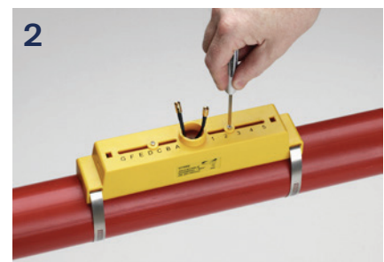
Clamp guide rail and sensor assembly to pipe and release sensor locking screws
