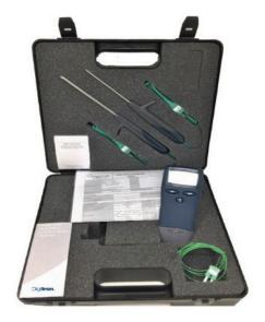
The immersion probe should be placed in the water to a minimum depth of 25mm; the surface probe may be used to take the temperature of pipes and tanks, and the wire probe can be used to reach awkward places or where the other probes are not appropriate. This kit comes with a traceable certificate of calibration.
